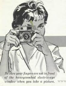
FOCUS THE CAMERA LENS by slowly turning the focus knob until the two range-finder images appear as one. The camera can be held either horizontally or vertically. If you prefer not to focus for each picture taken, you can set the focus knob to the symbol (▼) between 3 and 4 which is the setting for universal focus (15 feet).
