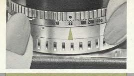
This simple adjustment sets the automatic exposure system for your film. Press the tab as shown and turn the film speed ring to the correct speed (ASA Exposure Index) of the film you are using. This adjustment is automatically locked by releasing tab.
